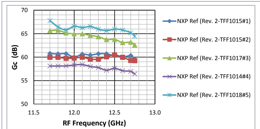
Fig 15. Conversion gain measurement results (High band/Horizontal)
