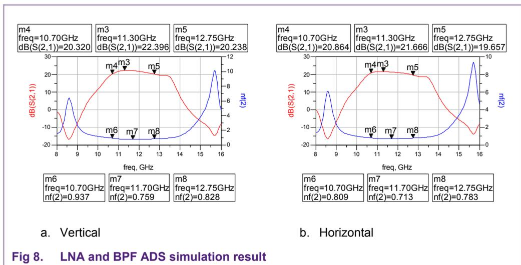
Fig 8. LNA and BPF ADS simulation result
