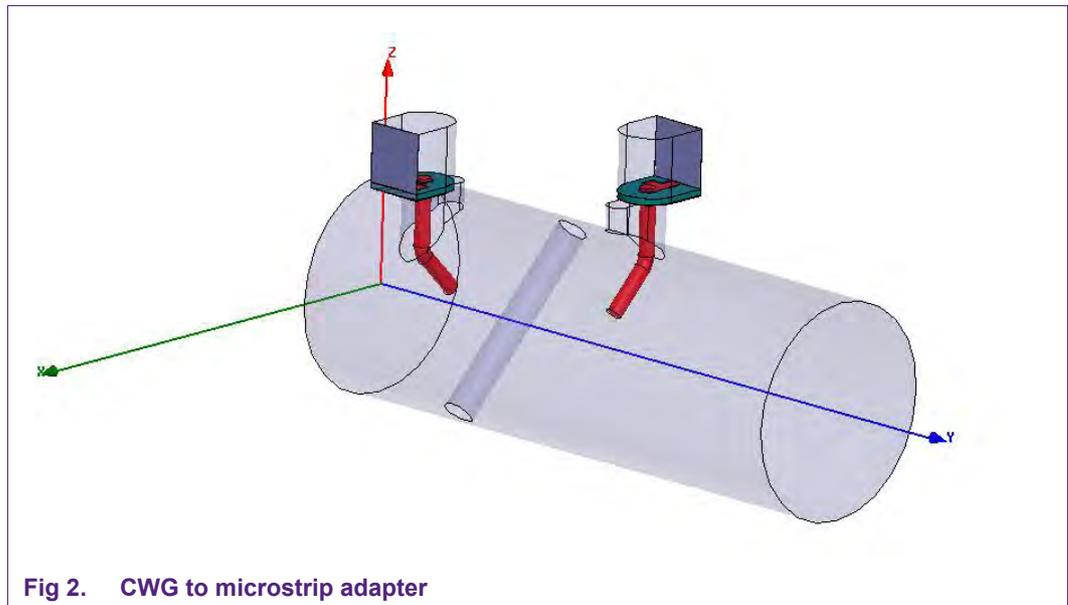
The drawing of the base (including a short stick) and probes are shown in Figure 3 and Figure 4 respectively, and the dimensions of the CWG, probe and probe holes are based on the dimension in the model in Figure 2. It is also important to assemble the probe with right direction and position. To solder the probes precisely, a fixture is designed to position the probes during soldering, and the assembly process is shown in Figure 5.
