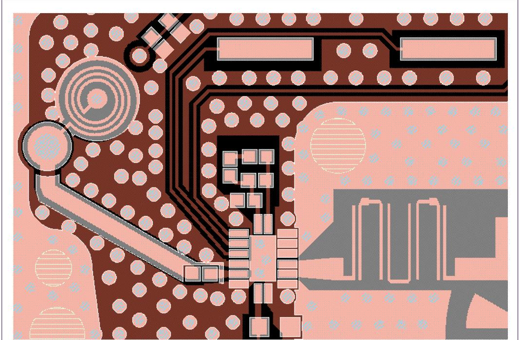
**Fig 9. The footprint of TFF101x and surrounding circuits**
