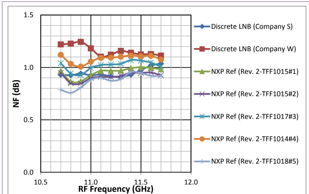
Fig 17. Noise figure measurement results (Low band/Horizontal)
