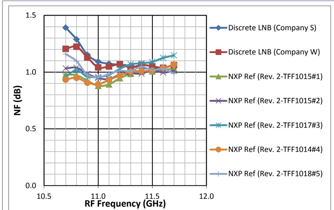
Fig 16. Noise figure measurement results (Low band/Vertical)
