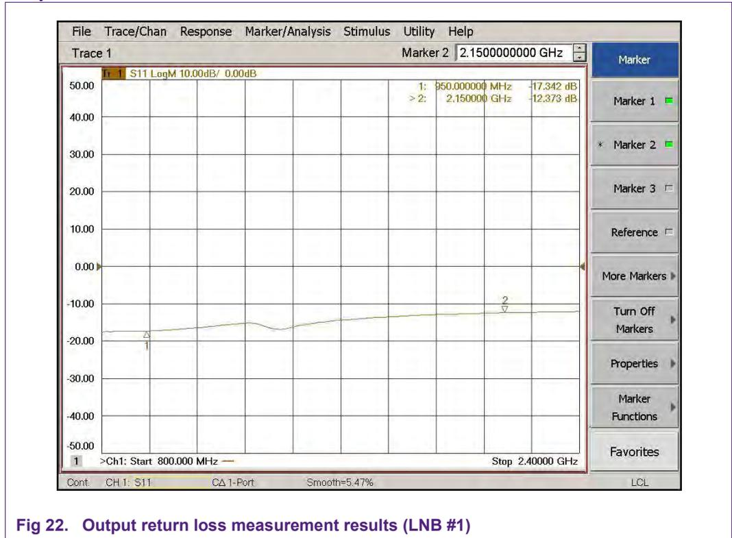
Fig 22. Output return loss measurement results (LNB #1)
