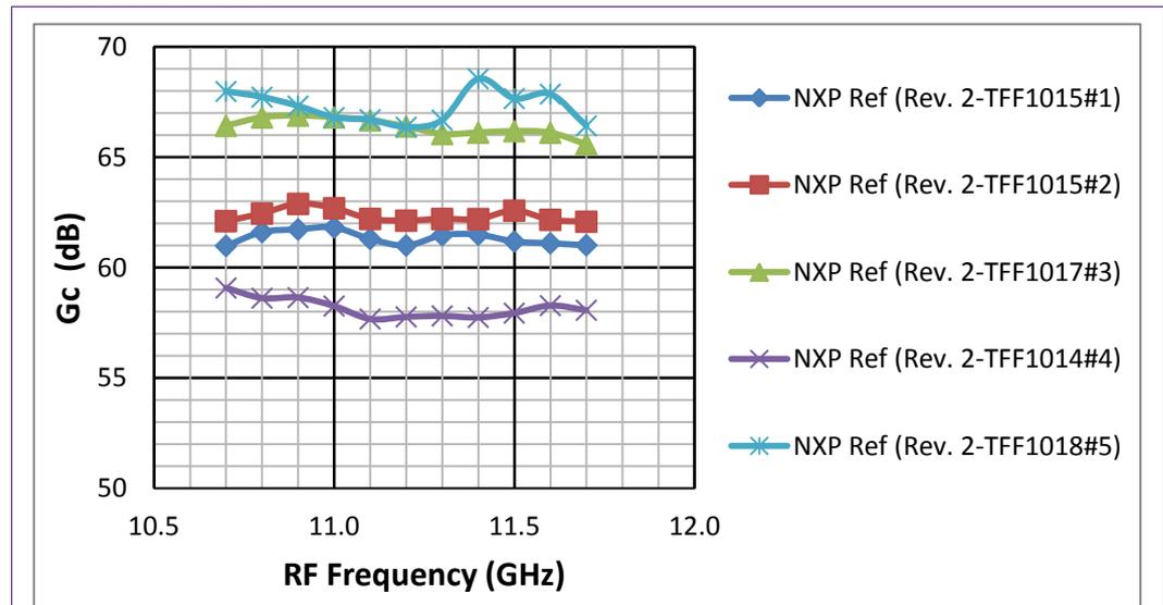
Fig 12. Conversion gain measurement results (Low band/Vertical)
