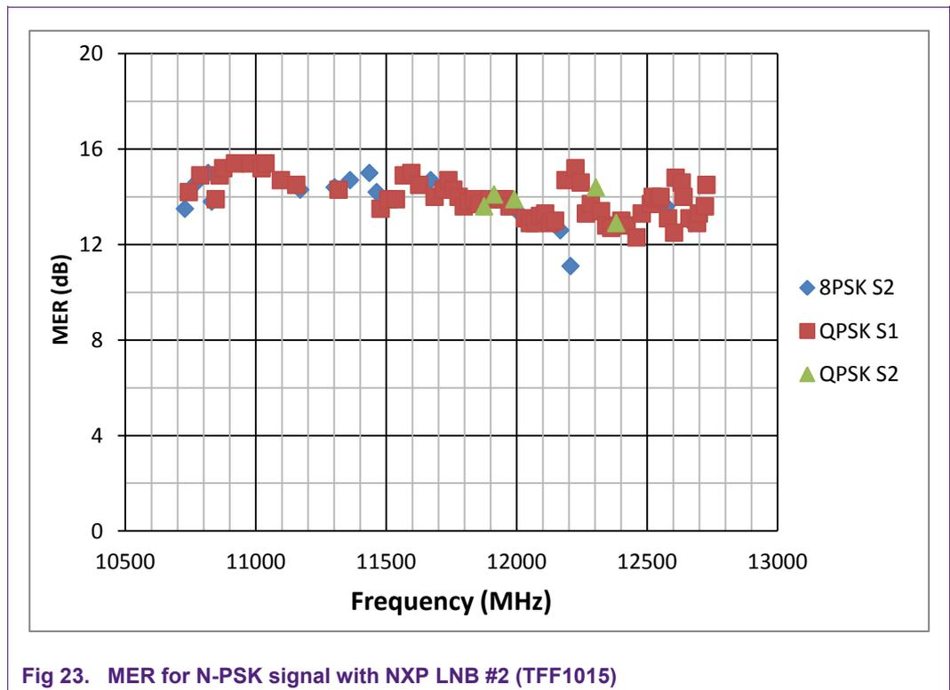
Fig 23. MER for N-PSK signal with NXP LNB #2 (TFF1015)
