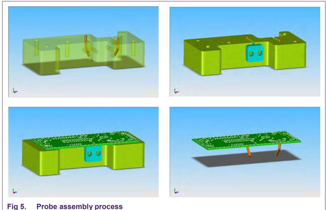
Fig 5. Probe assembly process
