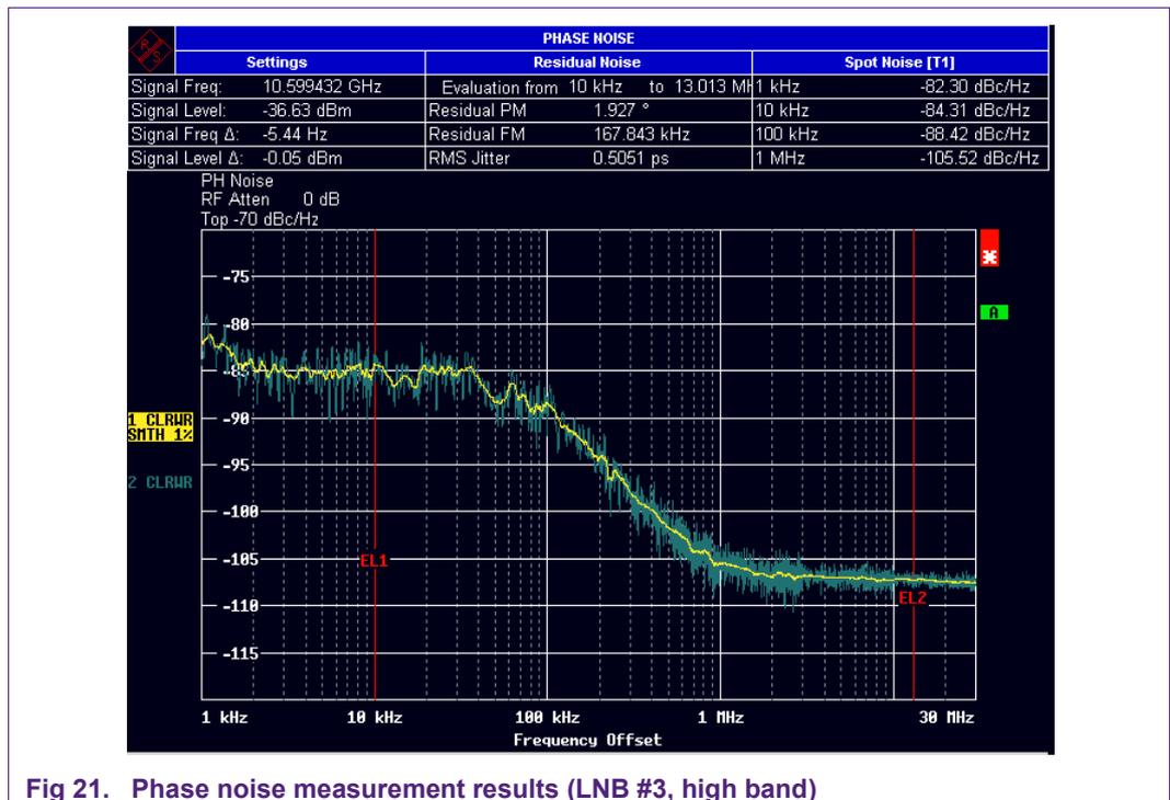
Fig 21. Phase noise measurement results (LNB #3, high band)
