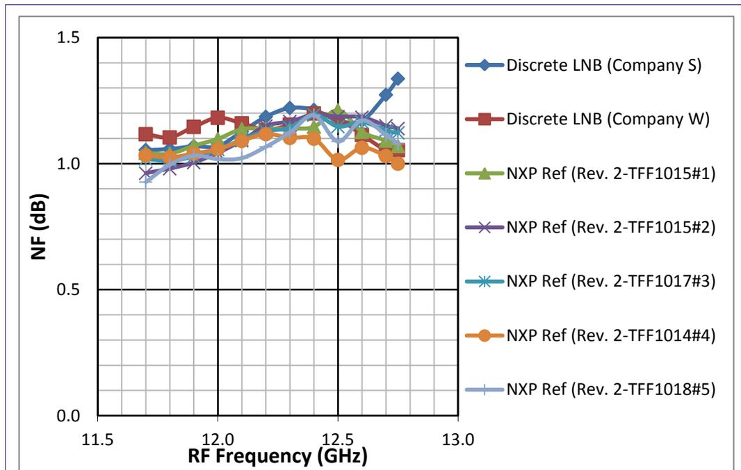
Fig 19. Noise figure measurement results (High band/Horizontal)
