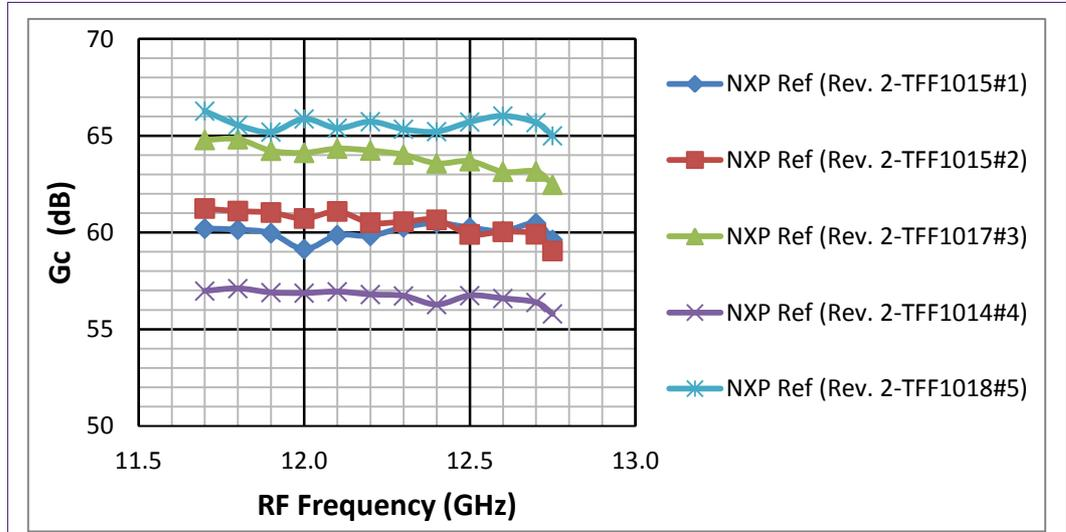
Fig 14. Conversion gain measurement results (High band/Vertical)
