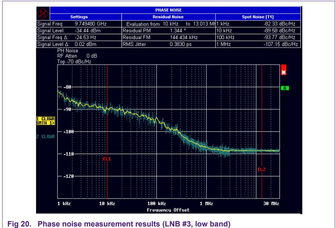
Fig 20. Phase noise measurement results (LNB #3, low band)
