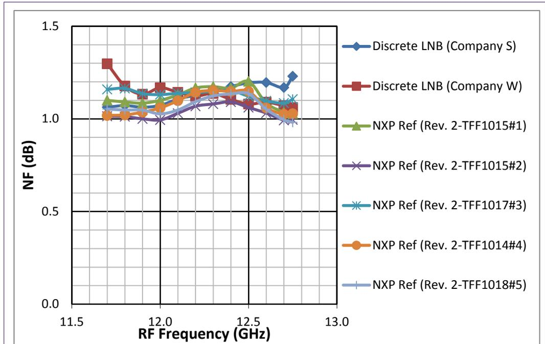
Fig 18. Noise figure measurement results (High band/Vertical)
