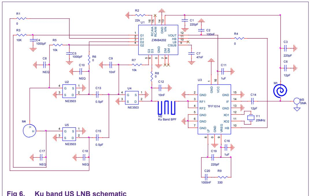
Fig 6. Ku band US LNB schematic
