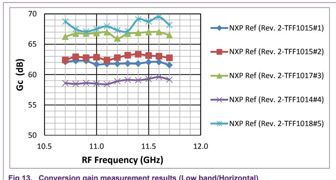
Fig 13. Conversion gain measurement results (Low band/Horizontal)
