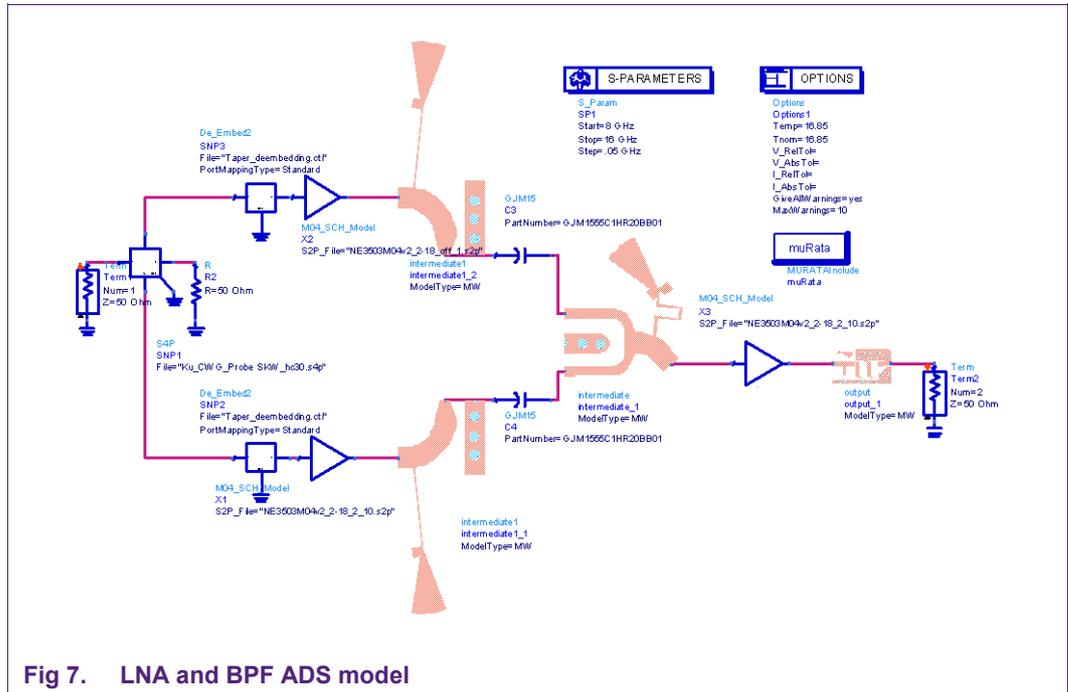
Fig 7. LNA and BPF ADS model
